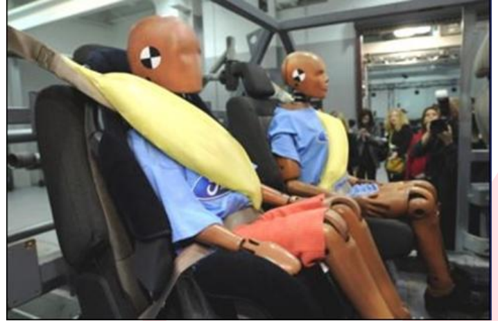
Inflatable seat belts Image courtesy of the Ford Motor Company
